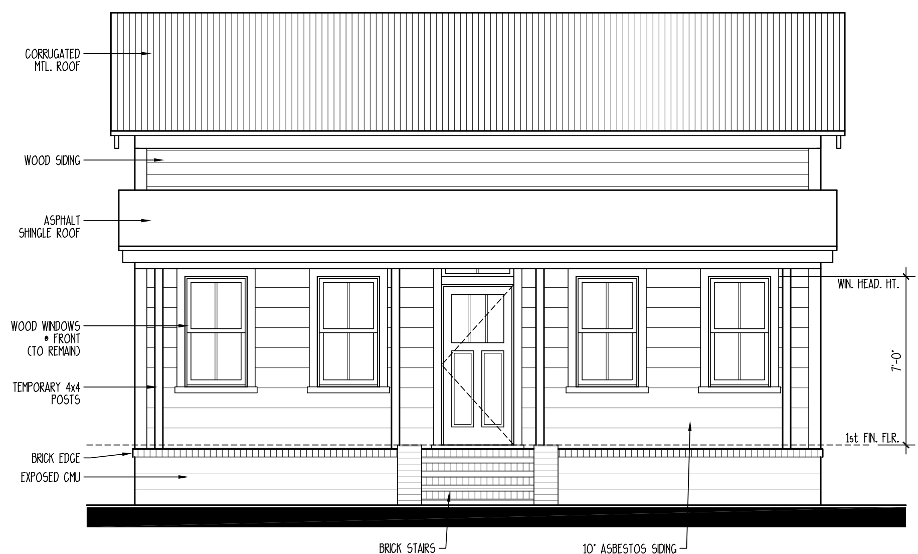
1 EXISTING FRONT ELEVATION
